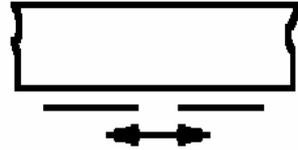
A schematic diagram of sliding doors. It shows a horizontal rectangle representing the door, with two horizontal lines below it and a double-headed arrow indicating the sliding mechanism. |
